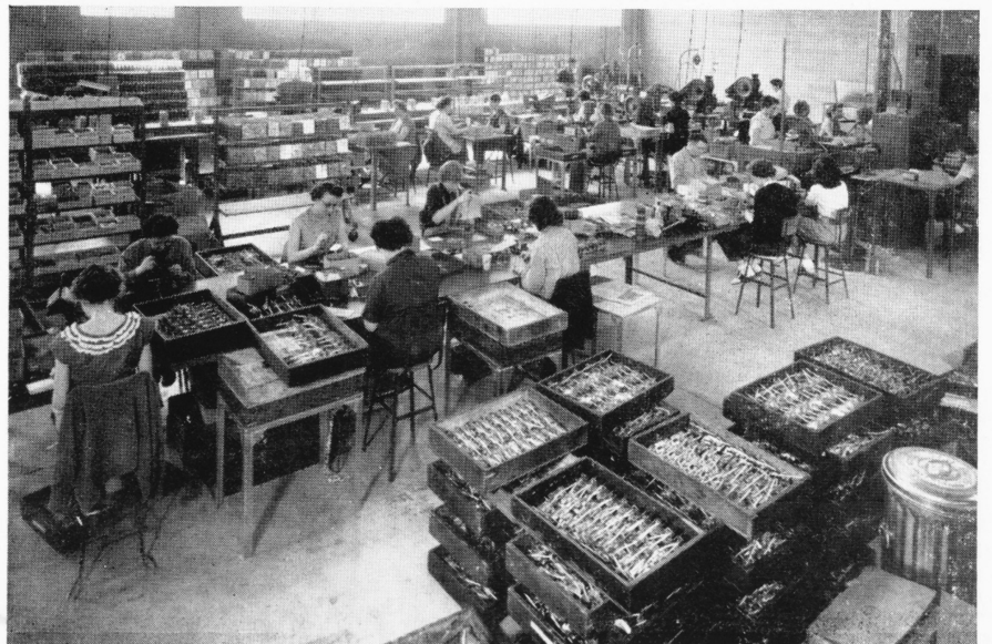
Assembling the internal mechanism of the toaster Chrome finish is applied in Udylite fully automatic machine (not shown)
